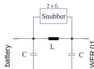
To smooth down the input sine current ( $2 \times f_0$ ), which is caused by very high input capacity a ch<sub>o</sub>ke can be connected input sided.
