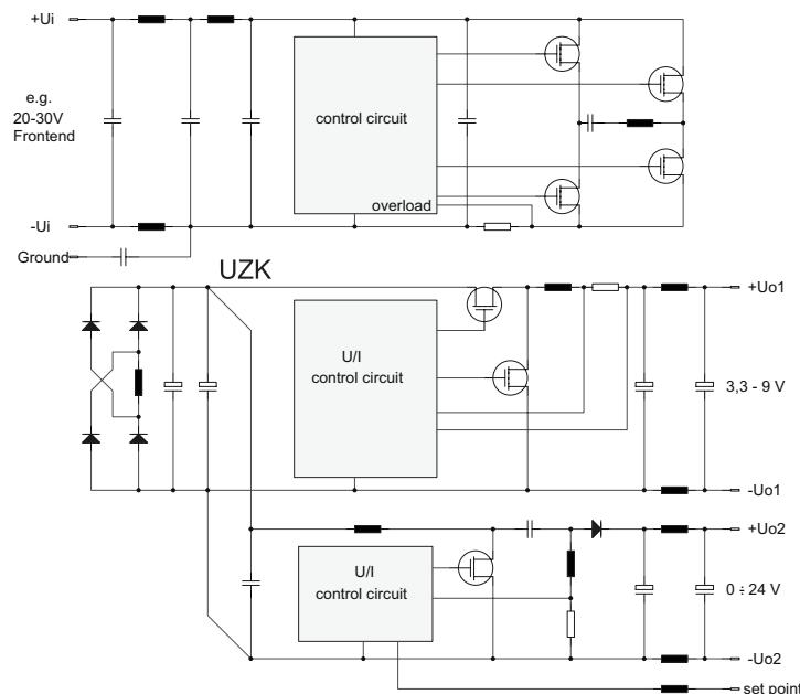
Instead of the synchron buck-regulator the patented Regenerator topology can be used to generate an adjustable output voltage from zero up to higher than the intermediate voltage. Corresponding mechanical adaptation, thermal coupling, EMC-capability and customer specification performance lead to a system suitable converter concept. With a timing processor the switch-on points of the single outputs can be defined.
