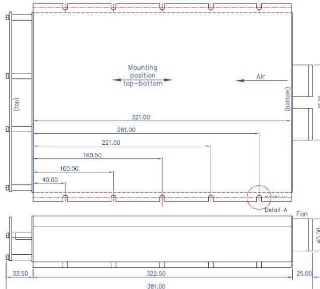
The fans must be placed in the bottom position to realise sufficient ventilation when the BOS Series is mounted.
